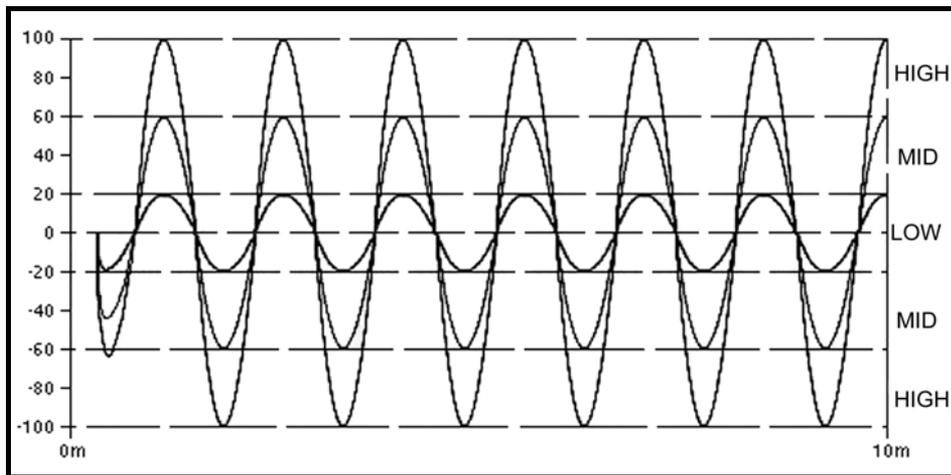
Figure 7.5: Sound waves with different amplitudes but same frequency
