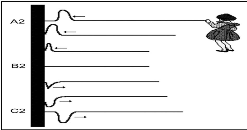
Figure 7.3: Movement of a transverse wave (Reprinted from *Encyclopedia Encarta* 2004 © 1993-2003 Microsoft Corporation).
